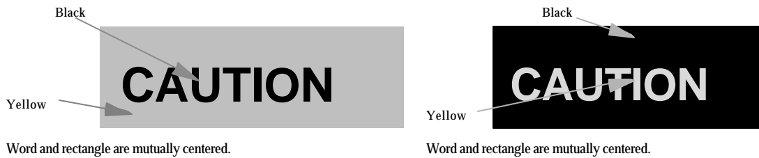
Figure 10—“CAUTION” sign for damage or interference without any safety impact
