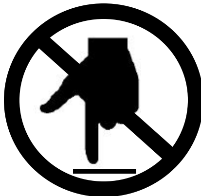
Figure 5—Use of circle and bar to show that an action is prohibited
